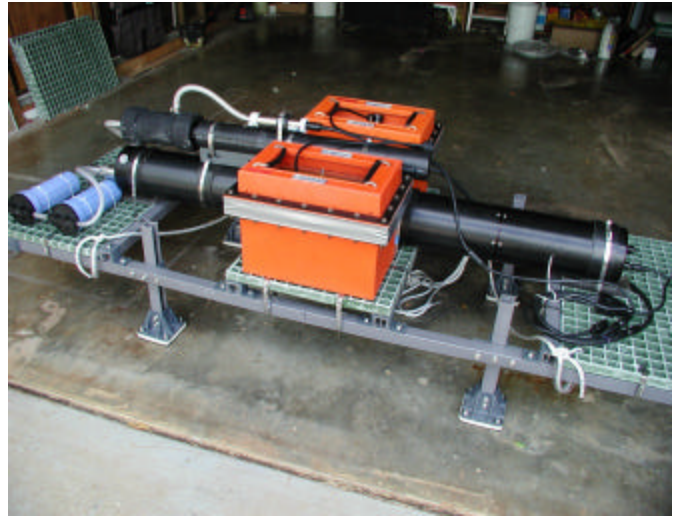
Fig. 8. Photograph of Mass SURFER, OS 200 CTD, Seabird pump, filtration cartridges and two 86 amp-hr external deep-sea batteries. The deployment frame is designed for a single-point lift.
