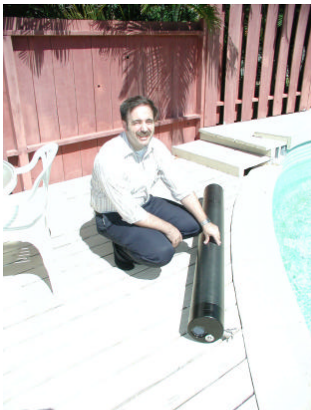
Fig. 1. Mass SURFER prototype prior to pool test. JPL scientist for scale. The pressure housing is 6.5 in. OD by 5.5 feet total length.
